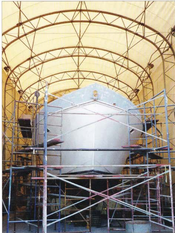
Due to limitations on new buildings built within 100' (30.4m) of the high-water mark, many of KKMI's shelters for larger boats are temporary fabric-covered structures such as this one for a 1970s motor-yacht in for core repairs and a paint job.
